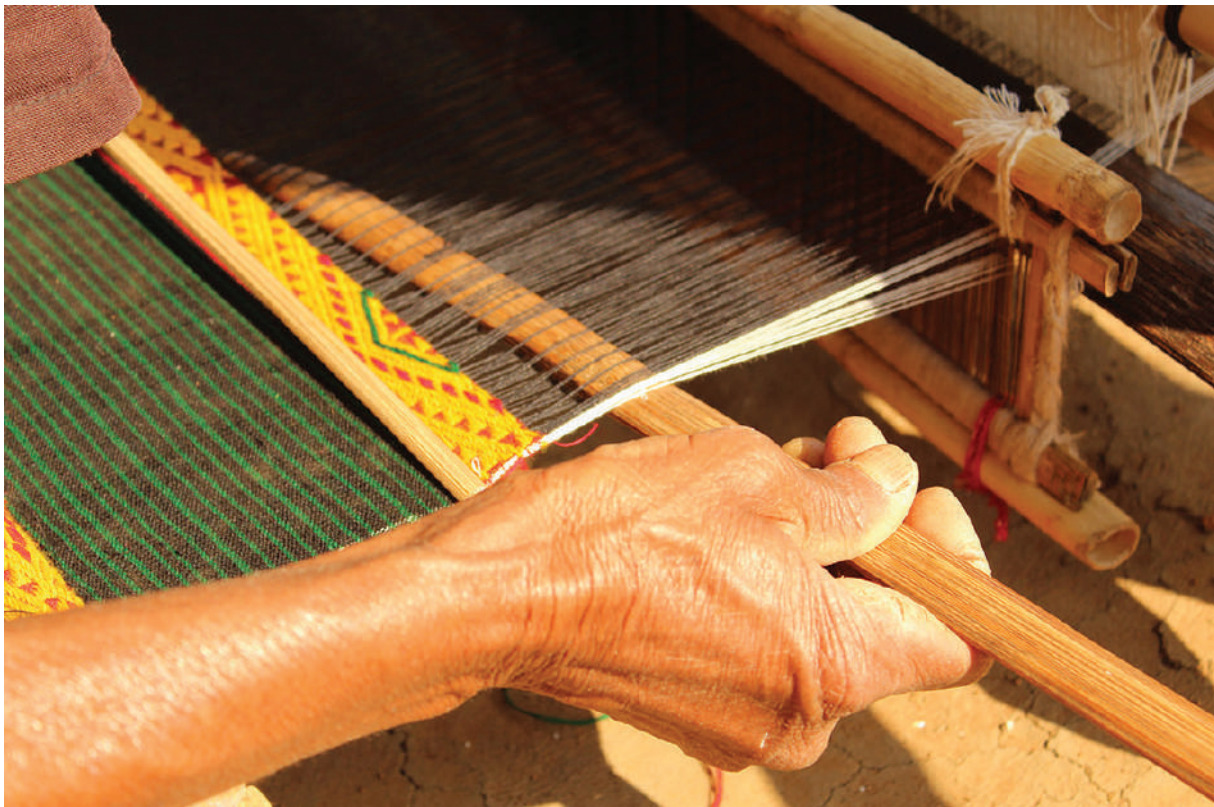
Figure 9: Picking the supplementary weft design with a smooth wooden sword.
