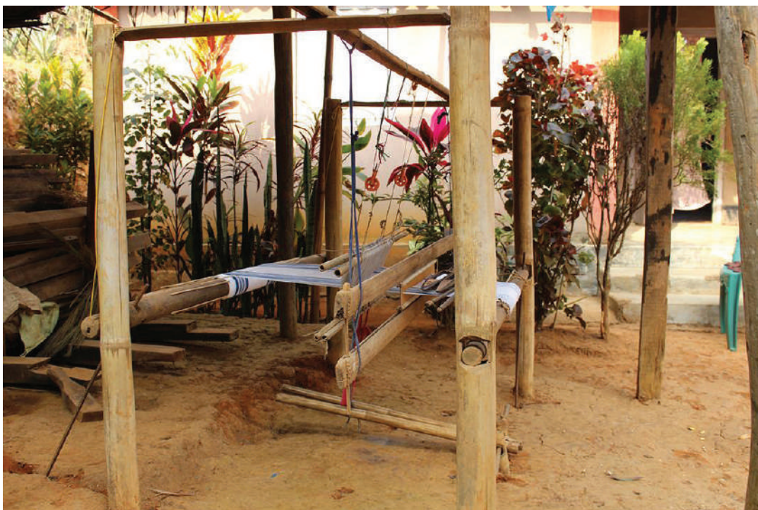
Figure 7: The thain ra of the Karbis of Plasha, a modified frame loom with shorter depth.
